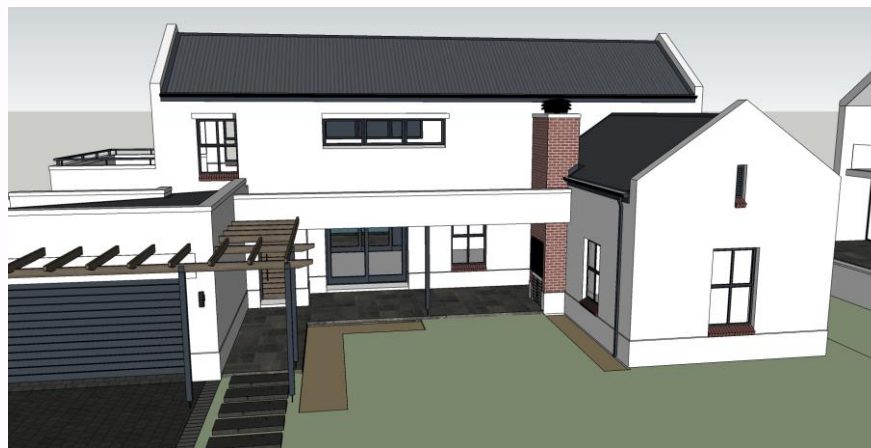
'Traditional' design with no cladding and parapet gable ends.
