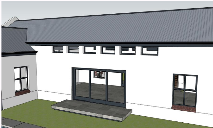
Clearstory windows in plastered wall (Single storey)
