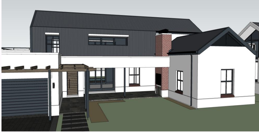
Wall cladding on double storey: Illustration of cladding and ‘eyebrow’ over windows. Fig. 4
