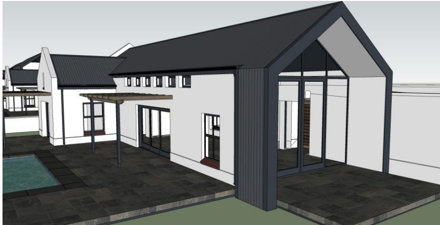
High volume-space. With clearstory windows, no eyebrows permitted. Fig. 5
