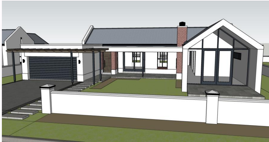
Pergola in front of garage and around to front entrance
