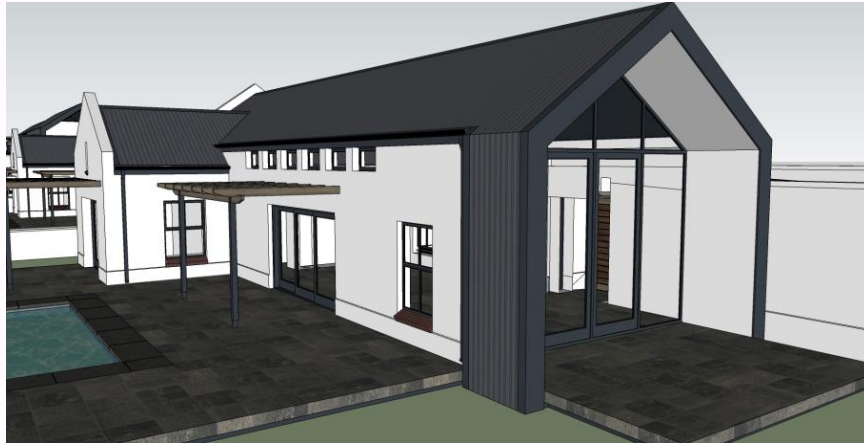
Gable-end, glazed and set back 1,5m min with partly cladded on the sides. Fig. 10
